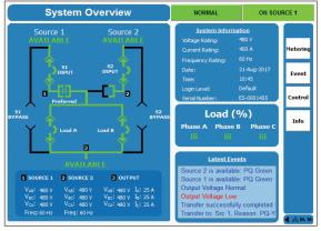
User-friendly control on all SS4 systems provide quick system configuration, power monitoring and response to alarms
