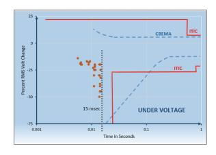
Figure 4: 60Hz data for critical loads meeting CBEMA/ITIC curves.
